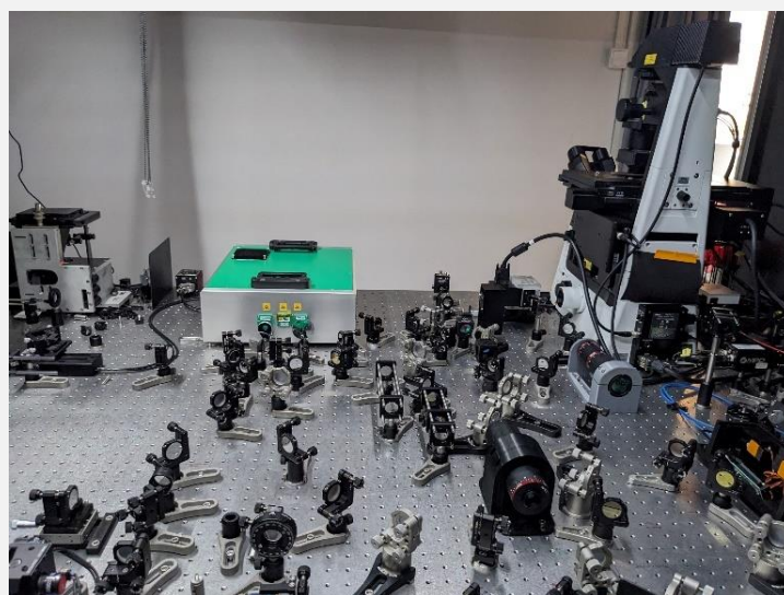
Figure 1: Prospective's FSX dual coupled in an optical path of an open table microscope. The fixe Stokes laser beam at 1030 nm was running over a time-delay (Thorlabs-Stage with movable mirrors) and the tunable Pump beam was set to 794 nm for label-free imaging of fat and lipids with wavenumbers at 2850\text{ cm}^{-1} .
