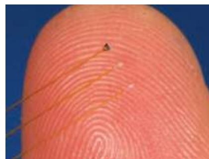
Figure 2. Fiber optic Fabry-Pérot medical pressure and temperature sensors. Courtesy of Abraham Katzir.
